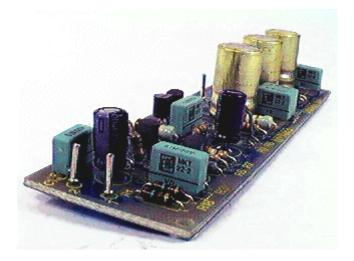
DO NOT use soldering flux apart from that which is already included in your solder. Too much flux can cause many problems and is one of the main causes of circuit malfunction. If nevertheless you have to use extra flux, as it is the case when you have to tin copper wires, clean it very thoroughly after you finish your work. In order to solder a component correctly you should do the following:
